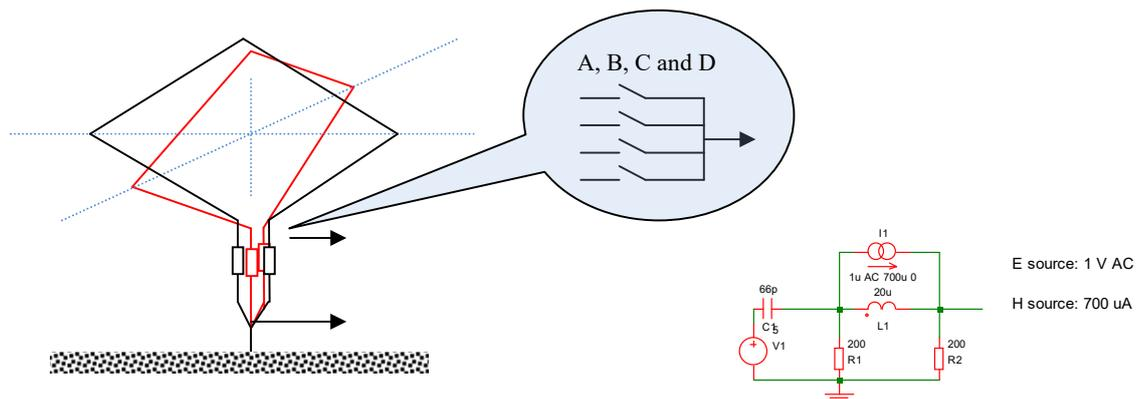
My antenna is realized in this way in an apple tree. According simulations the F/B-ratio is stable up to 4 MHz. **That is corresponding with my observations.**
