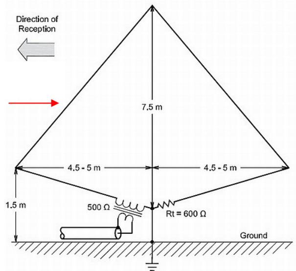
The operation is based on a well-known directivity effect, already used in airplane direction finding systems since the Second World War. The combination of a loop antenna and an E-field antenna make a cardioid directivity diagram with a sharp rear-side null. Just adding the signals of the two antennas is not enough. The requirements for a deep null are:
