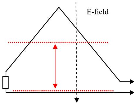
For the E-field conversion (in red) the conversion is equal to half the height of the structure, multiplied with the E field strength. This source has impedance  $C_{source}$  and is loaded with the resistor that connects the upper and lower part of the antenna.
