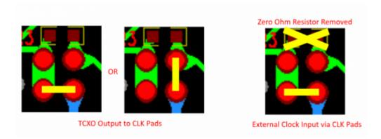
An example of CLK daisy chaining is shown below. One dongles TCXO is connected to two other dongles who have disconnected clocks.
