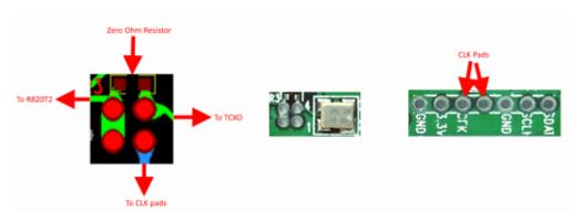
The first position allows you to output the dongles clock to the CLK pads. The second position allows you to input an external clock.
