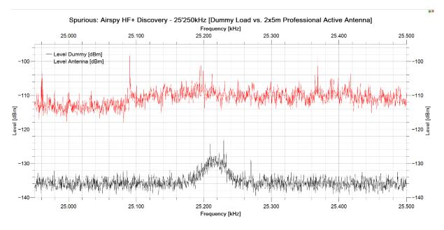
Here you see the usual spurious "hill" with a peak at -128dBm plus a very few distinctive peaks reaching up to -122dBm. With an antenna connected, the mean noise level rises from around - 138dBm to -114dBm in the lower frequency part to -112dBm [due to some local PV noise] in the upper part. Date/Time: August 28, 2019, 06:09 UTC.
