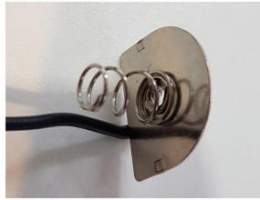
4. Install the terminals into the enclosure flat side down. You may need to use some force and light hammering to get it in.
