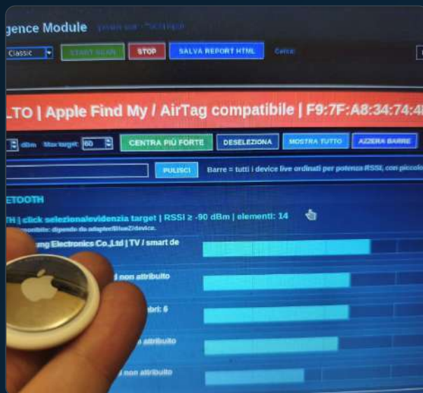
Live test with Apple Find My / AirTag-compatible alert shown on the Bluetooth module.
