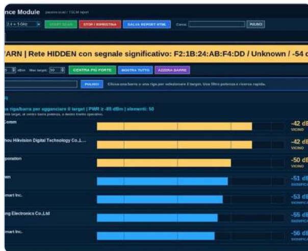
Wi-Fi Intelligence Module: AP/client visibility, hidden network warning and proximity bars.
