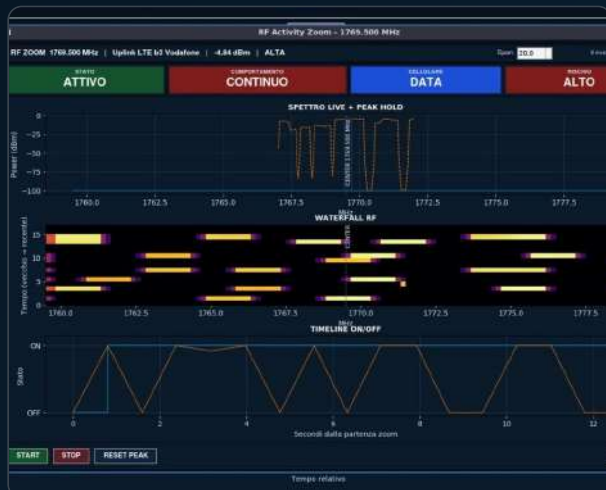
RF Zoom focused on an LTE uplink frequency: spectrum, peak hold, waterfall and on/off timing.
